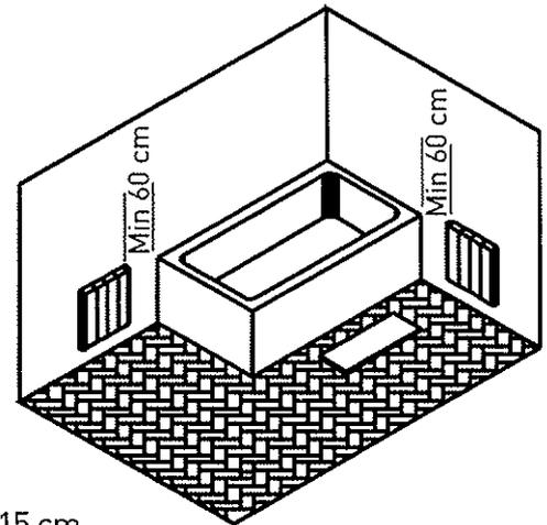
To avoid problems, it is necessary to keep a minimum distance of 15 cm between the radiator and any combustible material.
